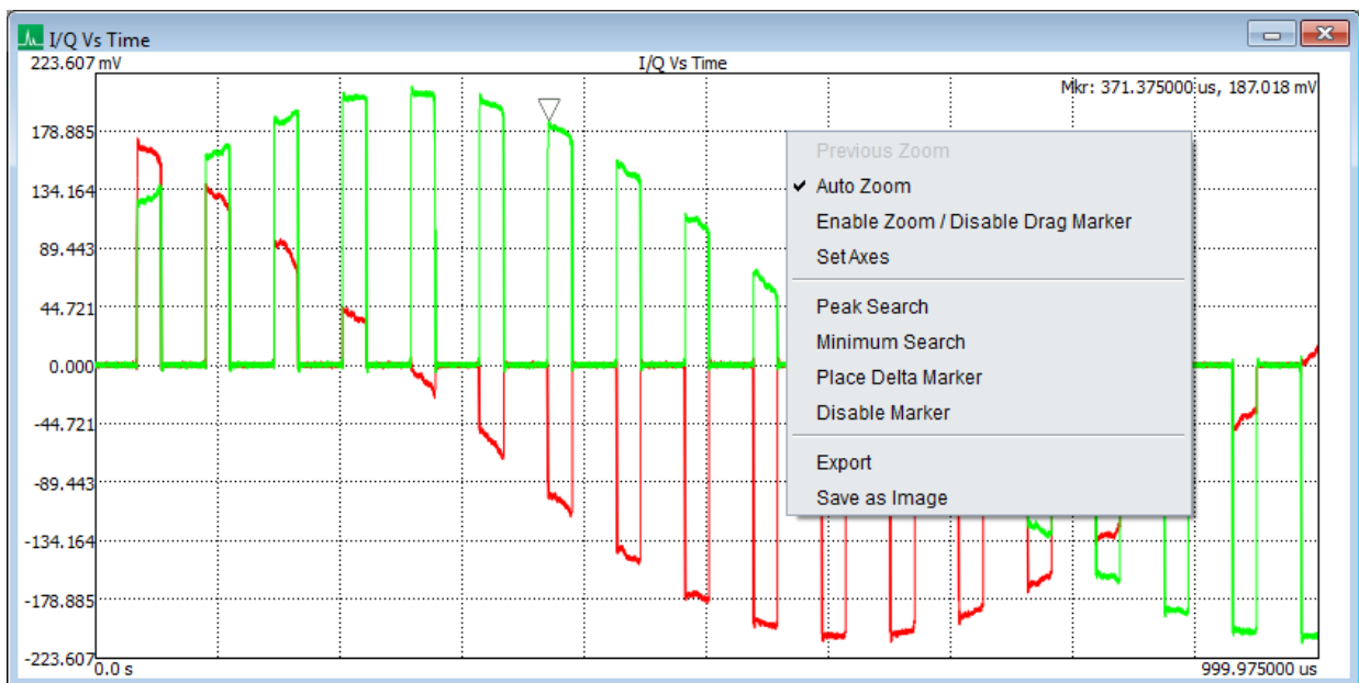
Figure 89: The context menu is displayed after right mouse clicking anywhere in the plot.
