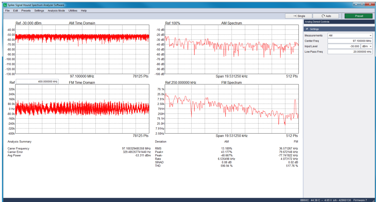
Figure 33: Viewing a broadcast FM signal and observing the 19kHz FM pilot tone in analog demodulation mode.
